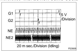
During cranking or idling check between ECM terminals G1, G2, NE and G≥, and between NE2 and NE2≥.
