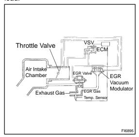
If even one of the following conditions is fulfilled, the VSV is turned ON by a signal from the ECM. This results in atmospheric air acting on the EGR valve, closing the EGR valve and shutting off the exhaust gas (EGR cut-off).
