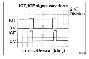
During cranking or idling, check waveforms between terminal IGT, IGF and E1 of ECM.
