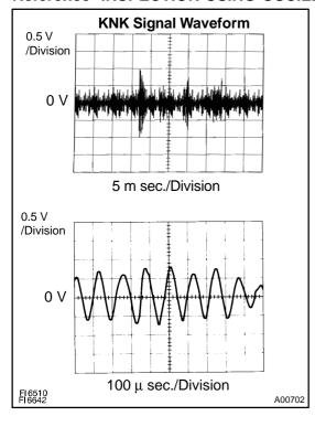
With the engine racing (4,000 rpm) measure waveform between terminals KNK1, KNK2 of ECM and body ground.
