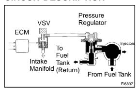
The ECM turns on a VSV (Vacuum Switching Valve) to draw the air into the diaphragm chamber of the pressure regulator if it detects that the temperature of the engine coolant is too high during engine staring.
