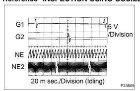
During cranking or idling check between ECM terminals G1, G2, NE and G≥, and between NE2 and NE2≥.
