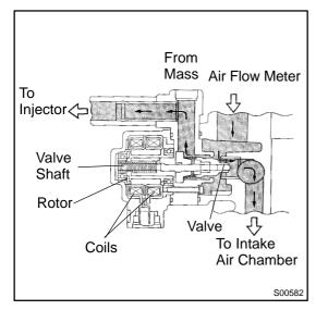
The step motor type IAC valve is located in front of the intake air chamber. Intake air bypassing the throttle valve is directed to the IAC valve through a passage. A step motor is built into the IAC valve. It consists of 4 coils, a magnetic rotor, valve shaft and valve.
